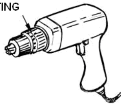
14 OR 18 VOLT CORDLESS DRILL OR ELECTRIC SCREW GUN W/ 5/16" SOCKET DRIVE (2500 RPM PREFERRED)
